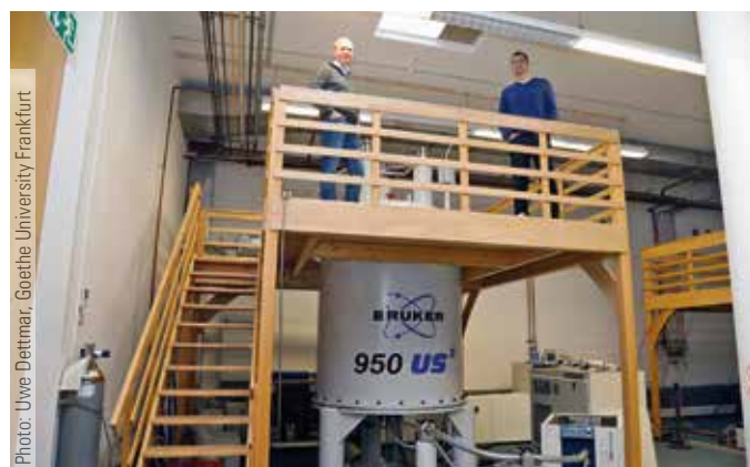
Dr Martin Hengesbach (left) and Dr Andreas Schlundt, NMR scientists from Goethe University, at the nuclear magnetic resonance spectrometer.
